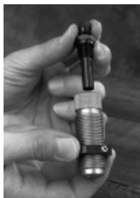
Seater dies in our 3-die sets use a "through-the-top" style seater plug as shown above. This allows for easy cleaning.
