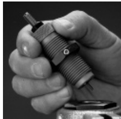
Screw the sizer die into the reloading press.
