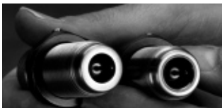
The standard RCBS steel die is shown on the left. The carbide insert is visible in the carbide sizer die on the right.
