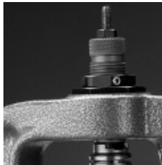
Notice the sizer die is adjusted so it contacts the shell holder.
