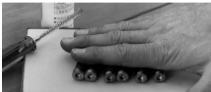
Roll cases on an RCBS Case Lube Pad for proper lubrication.
