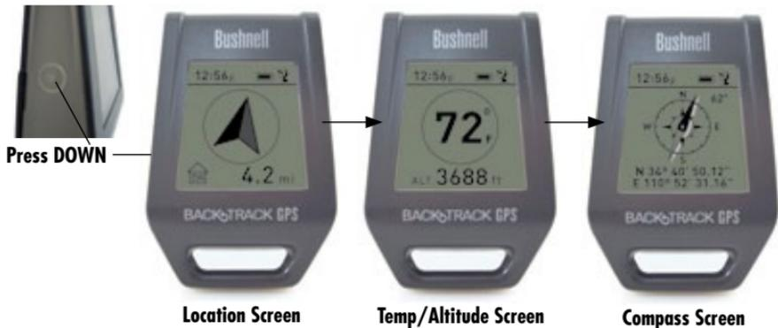
10. BackTrack Point-5 also provides two additional screens with useful information for outdoor enthusiasts. Press the **DOWN** button while on the **Location** screen. You will see a screen that displays the air temperature and altitude of your current location. Press **DOWN** again to view the **Compass** screen, which displays your current heading in degrees, minutes, and seconds.
