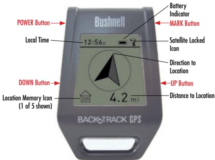
*Note: Control Buttons are located on the sides of the BackTrack*
