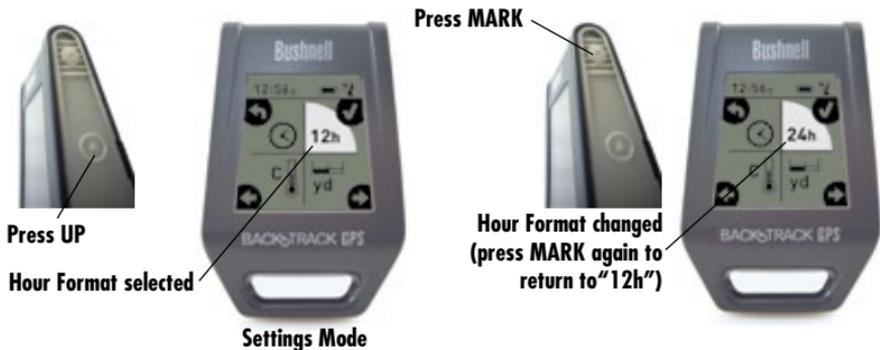
5. In **Settings Mode**, you may also change the other unit measurements. Press the **UP** or **DOWN** buttons to highlight the setting. Press the **MARK** button to change the unit measurement. You can change hour (12h to 24h), distance units (yards/miles to meters/kilometers), and temperature units (Fahrenheit to Celsius). Press **POWER** button to exit when done.
