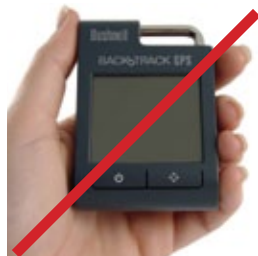
Incorrect Operating Position
